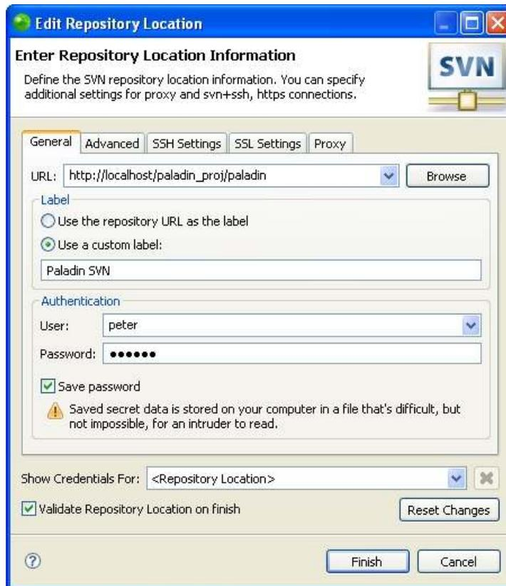
Figure 1 - Establishing a Connection to an SVN Repository Server.
